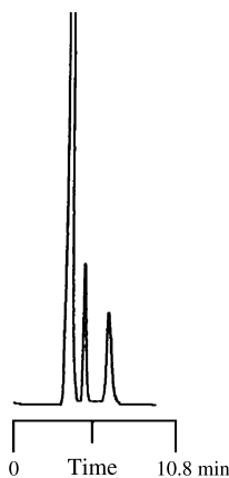
Fig. 3. Chromatogram showing the enantioresolution of FCC-pyroglutamic acid on a teicoplanin bonded chiral stationary phase using the methanol phase of 95 MeOH/5 EE/0.2 HOAC/0.4 TEA by volume (v/v). To the best of our knowledge, pyroglutamic acid is resolved in derivatized form for the first time under the elution of non-aqueous mobile phase
